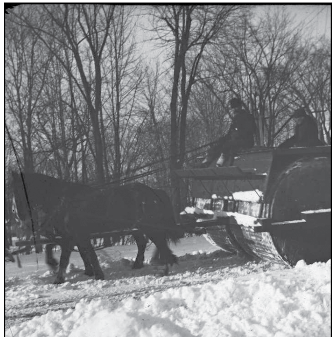
A horse-drawn snow roller in Brunswick, 1897. George J. Mitchell Department of Special Collections & Archives, Bowdoin College Library.
